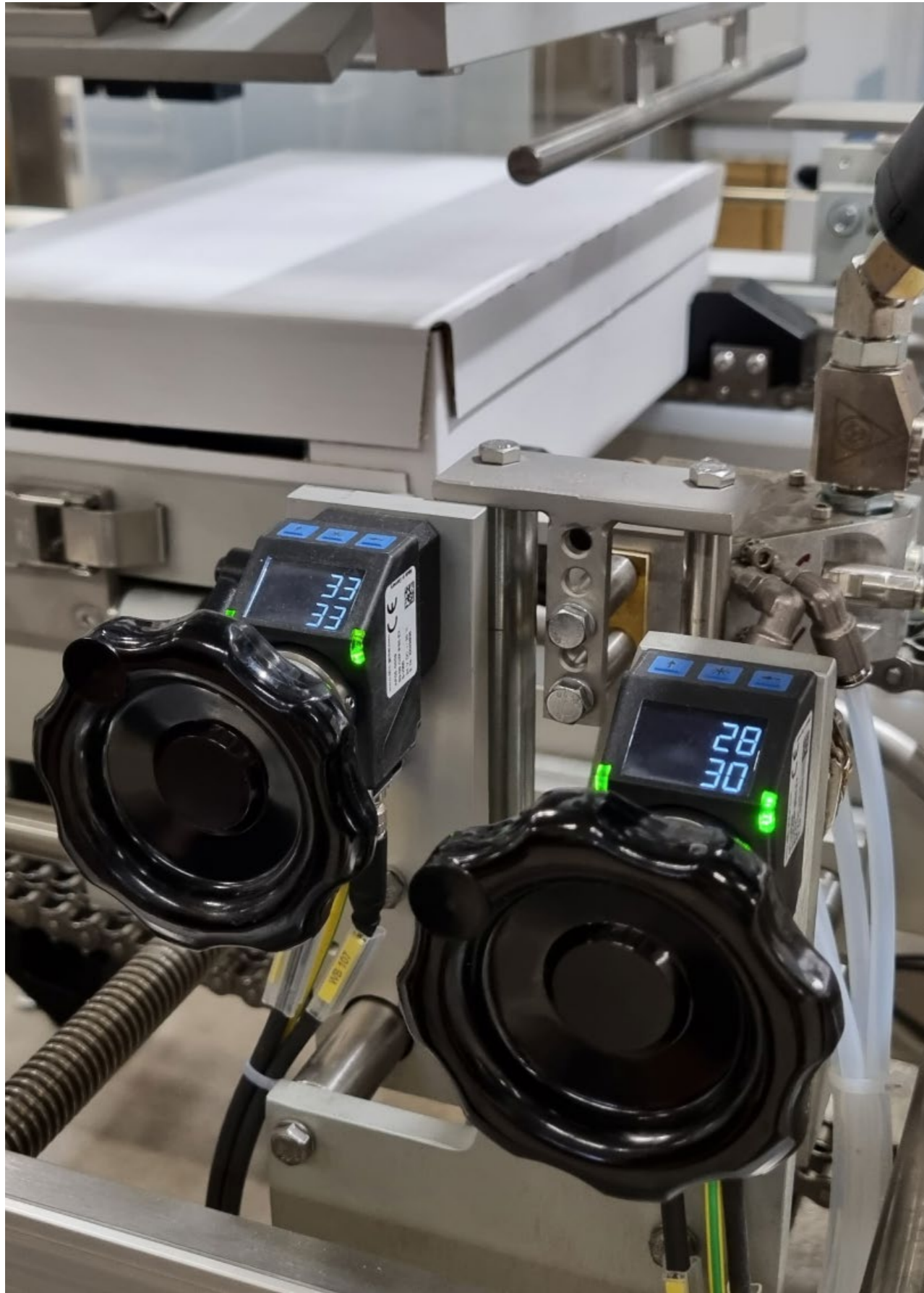
Optional digital display for efficient adjustment of the machine
